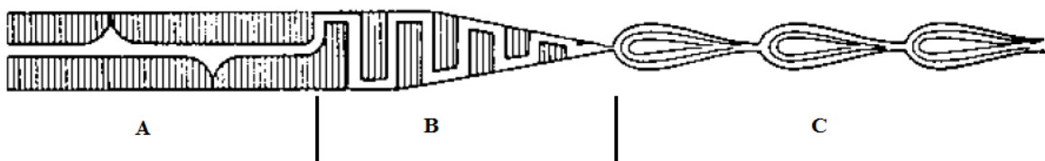
Figure (2-3) Shows diagram of stages of cracking into amorphous polymers. Region A: crack advance by void creation; region B: crack advance along alternate craze–matrix interfaces; region c: crack advance through craze bundle to form hackle bands [58].
