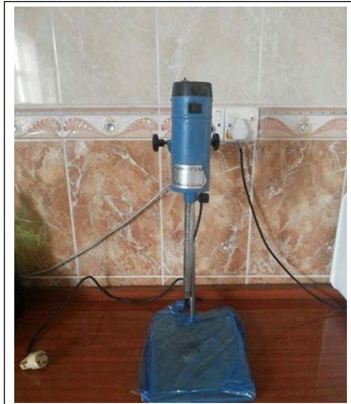
Fig.(3-3) Homogenizer (50Watt, 23KHz, 110Volt)
