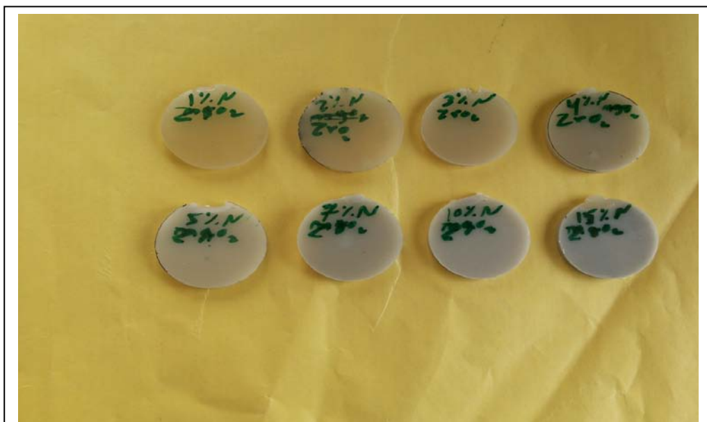
Fig. (3-6). Final epoxy and epoxy nano/microcomposite samples shape prepared for dielectrical test
